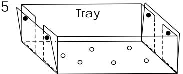
Fold the trough and put the rivets to make the tray.
